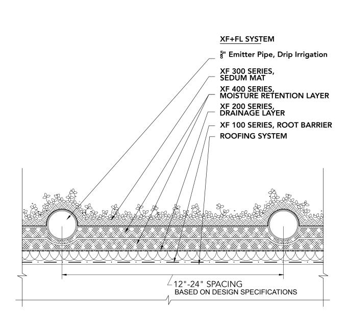
NOTE: 1- INSTALL THE ROOT BARRIER DIRECTLY ON TOP OF WATERPROOFING MEMBRANE.
