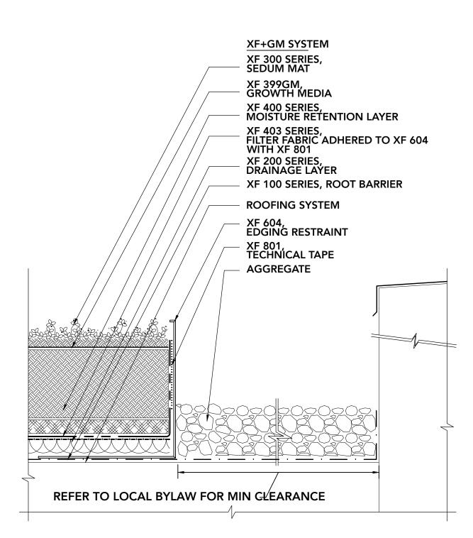
NOTE: 1- INSTALL THE ROOT BARRIER DIRECTLY ON TOP OF WATERPROOFING MEMBRANE.
