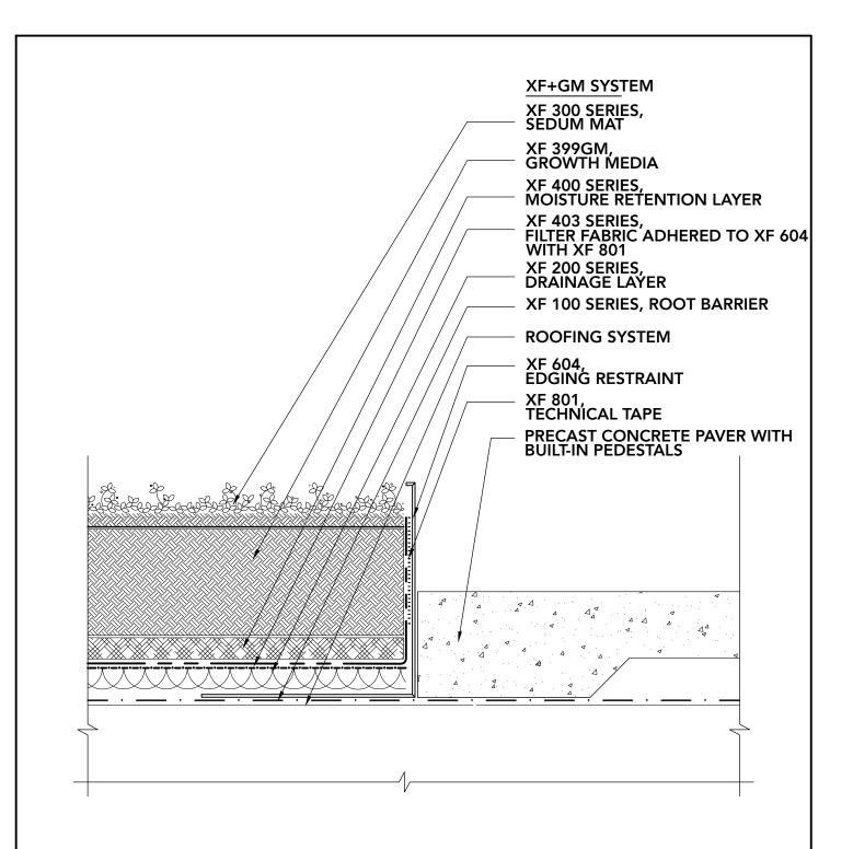
NOTE: 1- INSTALL THE ROOT BARRIER DIRECTLY ON TOP OF WATERPROOFING MEMBRANE.
